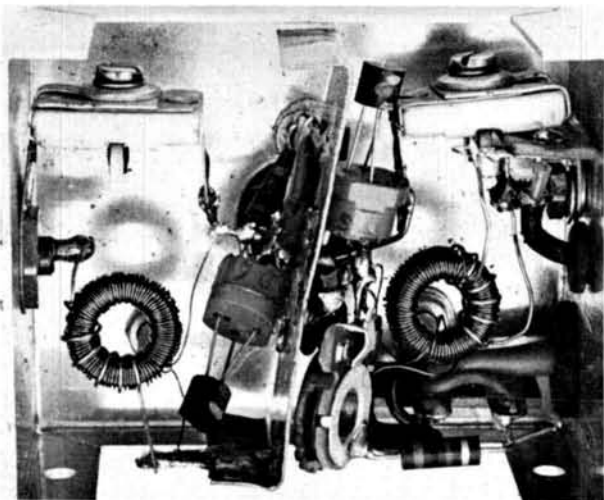
Cascode amplifier used for gain redistribution is installed in a small enclosure. The shield must be in place between the stages of the amplifier.
