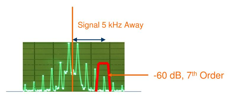
IF Filter vs. Adjacent Signal and IMD Splatter
